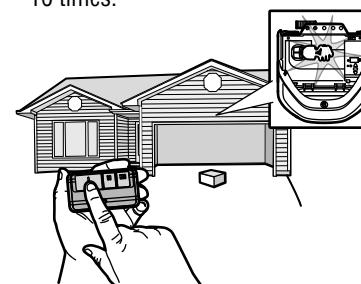
The garage door opener will not close from a remote control if the LED in either safety reversing sensor is off (alerting you to the fact that the sensor is misaligned or obstructed).
