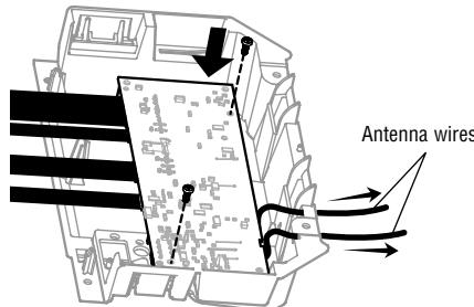
*NOTE: Some models will require the short antenna wire to be placed in the traps of the end panel.*
