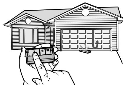
If the door stops and does not reverse on the obstruction, increase the down travel (refer to Adjustment Step 1).
