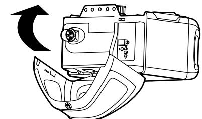
*NOTE:* When installing the light lens, ensure the antenna wires are hanging straight down.
