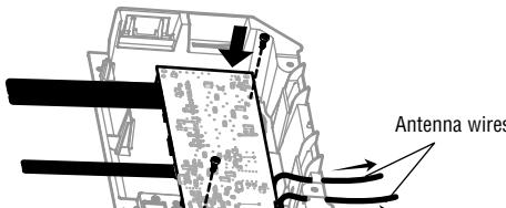
*NOTE:* Some models will require the short antenna wire to be placed in the traps of the end panel.
