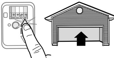
*NOTE: The UP and DOWN Buttons can be used to move the door up and down as needed.*
