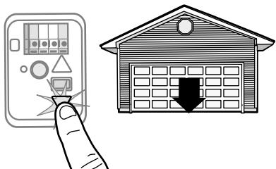
*NOTE: The UP and DOWN Buttons can be used to move the door up and down as needed.*
